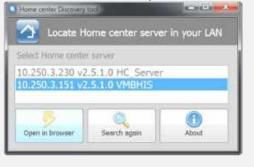
**4.** You can also enter the IP address of your HIS v2 directly into the **browser's address bar**. You can use this IP address retrieval via the iPhone/iPad app via the WIFI connected to the network in which the Home center module is located: the IP address appears automatically in the application. Or via the Home center client on Windows, this can be seen on the login screen.
