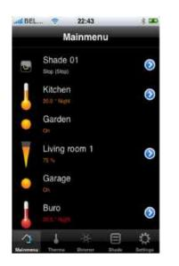
Home center for iPhone lets you operate and monitor all controls of your system. On connection, all available controls are downloaded to your iPhone. Each control can be operated by tapping it. The result of your action will immediately be visible in your house (for instance light goes on) and in the iPhone app (icon will be lit).
