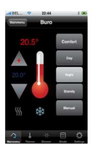
In the list, thermostats are displayed as an item with a thermometer and its name next to it. You can also read the current temperature and the active regime.
